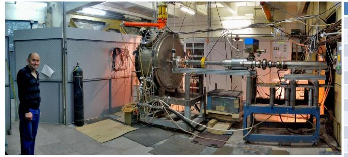
RF Gun Features: Gridded thermionic dispenser cathode driven by special modulator with GaN rf transistor;
