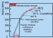
Stress-strain curves at 77 K for biaxially streched PEN films with various degrees of crystallinity.[2]
