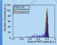
PEN light yield claimed by [1] could be reproduced by replicating the original setup using large surface PMT. The difference in light collection efficiency observed in the spectrometer setup is attributed to lower attenuation length in PEN. Measurements were made at Lancaster University. [5]
