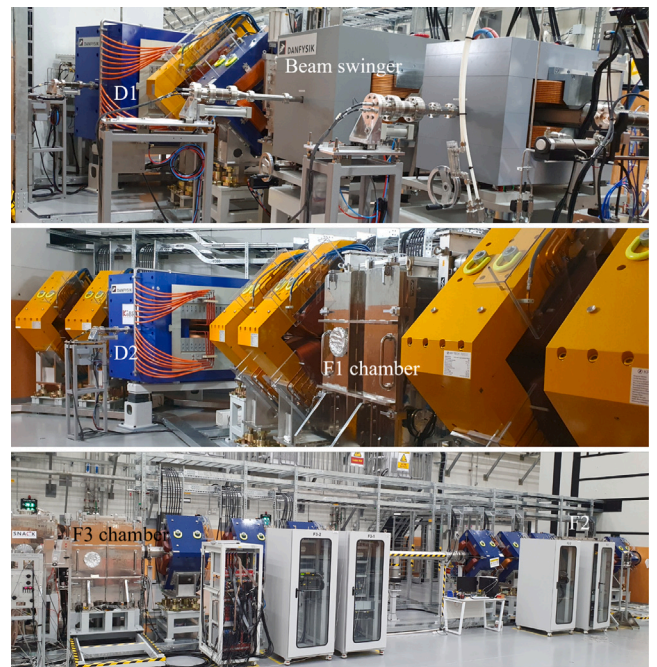
Fig. 5. Photographs of KoBRA. (top) Photograph around the production target. (middle) Photograph around the F1 chamber. (bottom) Photograph around the F3 chamber.
