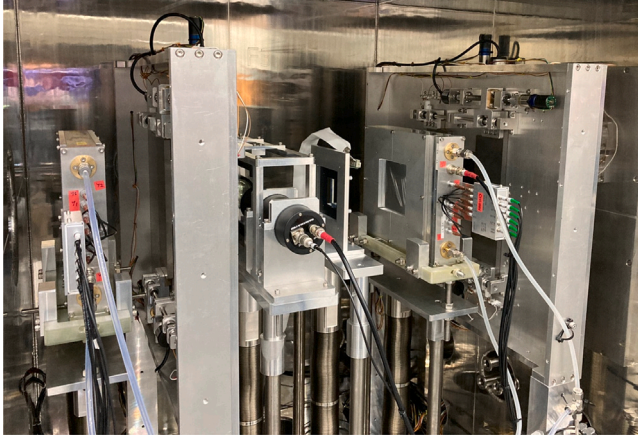
Fig. 6. Photograph of inside of the F3 chamber. The plastic detector, silicon detector, and small PPAC were installed between the slits.
