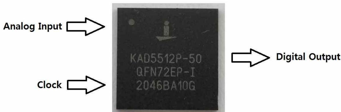
➤ We call Flash ADC(FADC) when ADC has sampling rate more than 10 MHz.
