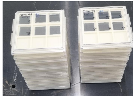
Thinning (by TRinno Tech) & dicing (by MEMSPACK)
