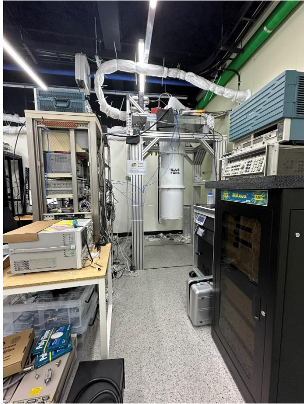
Dedicated Dilution refrigerator
