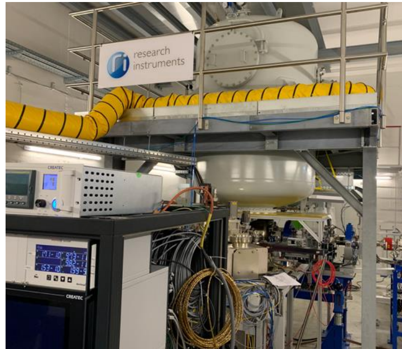
HV power supply suited for high bunch charge (designed for 40 mA, 450 kV)
