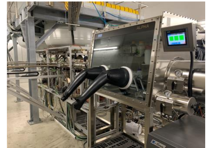
A Photocathode Preparation Facility (PPF)
