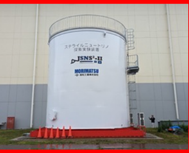
(JSNS 2 -II: New detector) 32t GdLS fiducial (6.2m dia. x 6.2m (h) ~230 10" PMTs)
