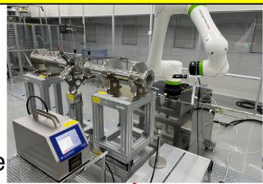
Robot arm for auto cleaning
