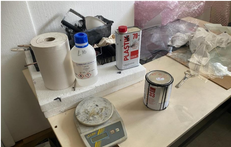
Carbon ink for HV electrode
