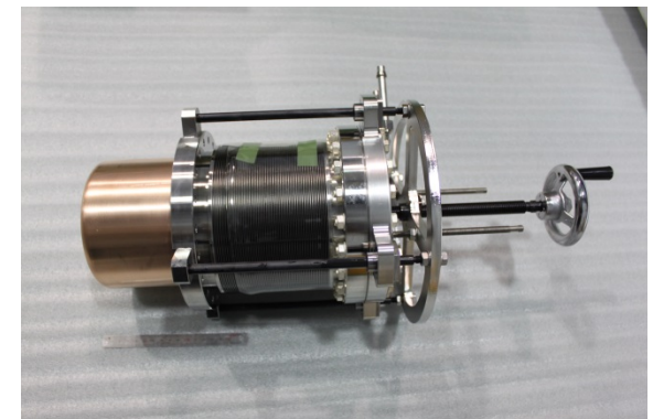
Movable slug tuner(stroke 90mm)
