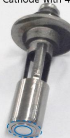
Cathode with 4.2 mm dia.
