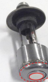
Cathode with 5.6 mm dia.
