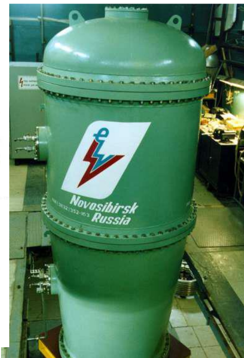
2.5 MeV, 100 kW Accelerator (EB-Tech)
