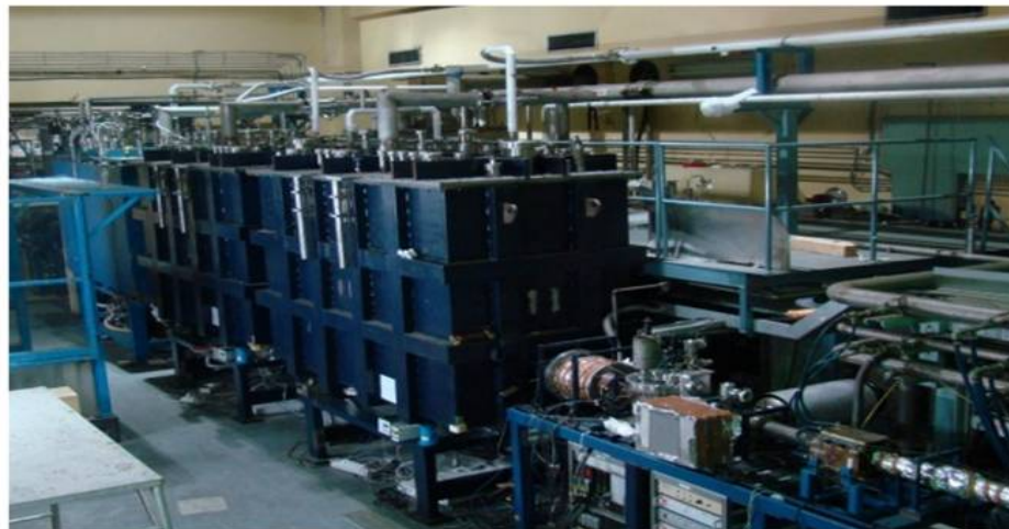
Nb QWR based Superconducting LINAC
