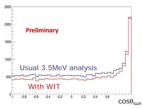
Preliminary study; A tighter <sup>16</sup>N cut makes reduction of the total number of BG by 20% with few % loss of signals.
