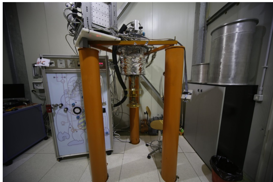
Completely customized Leiden dry 400 (6.8 mK) 2012
