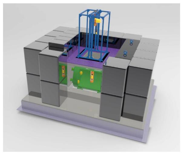
• The veto is composed by a tank, filled with ~2 ton of liquid scintillator, equipped with 10 Hamamtsu R5912-100 PMTs.
