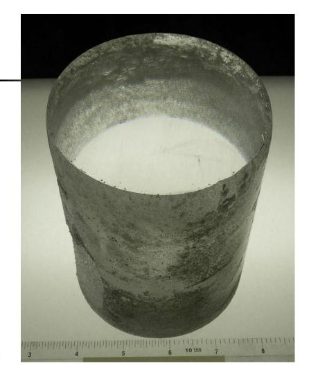
Target crystals are 4" in diameter and 8" in length (mass ~5 kg)
