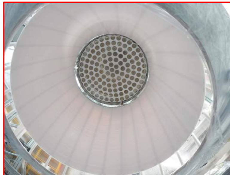
127 PMTs in the top array
