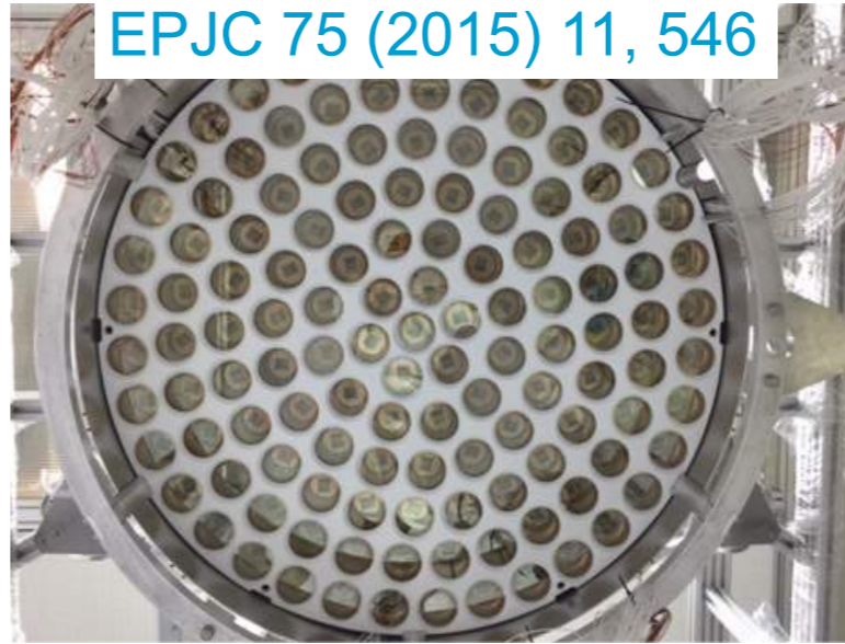
127 PMTs in the top array
