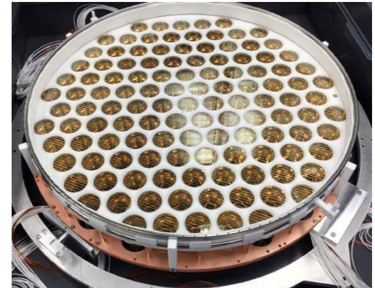
121 PMTs in the bottom array
