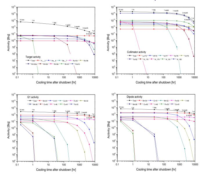
Decay gamma spectra were estimated at each component and cooling time step for evaluating shutdown dose rate.
