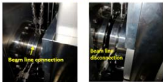
< Pillow seal test of TIS Module >
