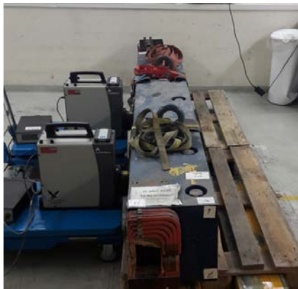
One of a series of in-situ gamma-spectrometry measurements performed on the “blue magnet”
