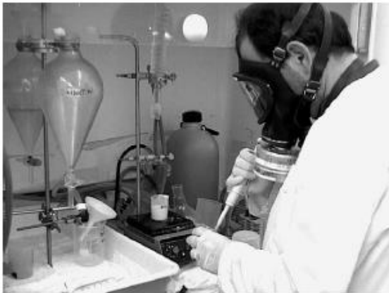
Fig.3. Addition of \text{Pb}(\text{NO}_3)_2 to the iodide solution to precipitate lead iodide.
