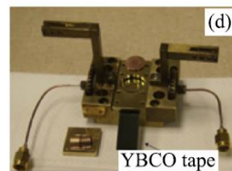
Figure 2. Schematic representation of (a) TE 016 mode 13 GHz BZT SiPDR and (b) TE 011 mode 9.4 GHz rutile RDR, designed to accommodate 12 mm wide tapes, are shown. SiPDR and RDR pictures are presented in (c) and (d), respectively.
