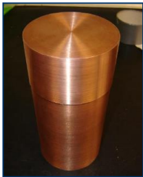
Housing made at LSC of electroformed copper
