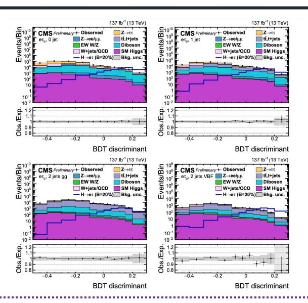
BDT discriminant distributions for the data and background processes in the H→et channel. A B(H→et) of 20% is assumed for the signal. The channel categories are 0 jets (upper row left), 1 jet (upper row right), 2 jets ggH (lower row left), and 2 jets VBF (lower row right). The lower panel in each plot shows the ratio of data and estimated background. The estimated background. The uncertainty band corresponds to the post-fit statistical and systematic uncertainties added in quadrature.
