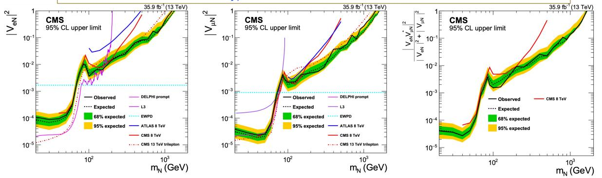
The search is sensitive to masses of N from 20 to 1600 GeV with 36fb<sup>-1</sup> of proton-proton collision data
