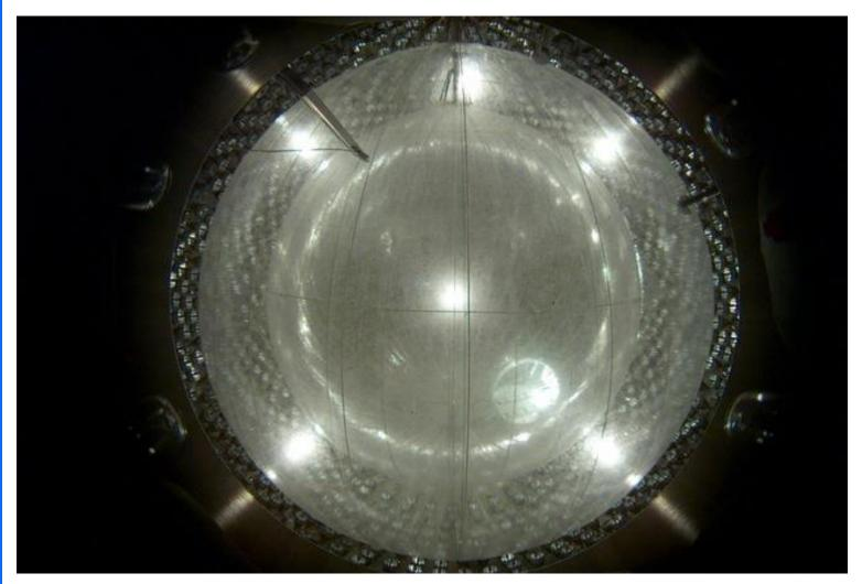
The nylon vessels were inflated in the sphere with synthetic air:  $C_{Rn} < 0.1 \text{ mBq/m}^3$
