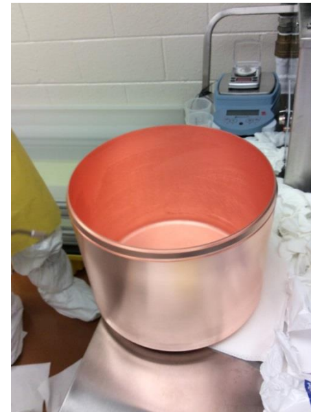
The cryostat containing the Ge detectors
