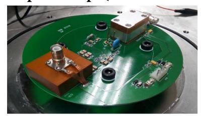
Silicon PIN photodiode (S3204-9,  $18 \times 18 \text{ mm}^2$ , Hamamatsu)
