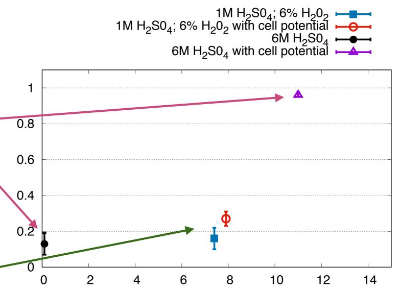
A cell potential alone can oxidize Po in an acidic environment - similar to standard electropolishing
