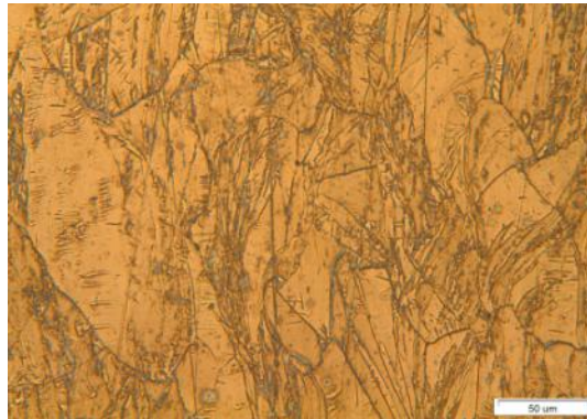
№2. 25% rolling, vacuum annealing at 700°C.
