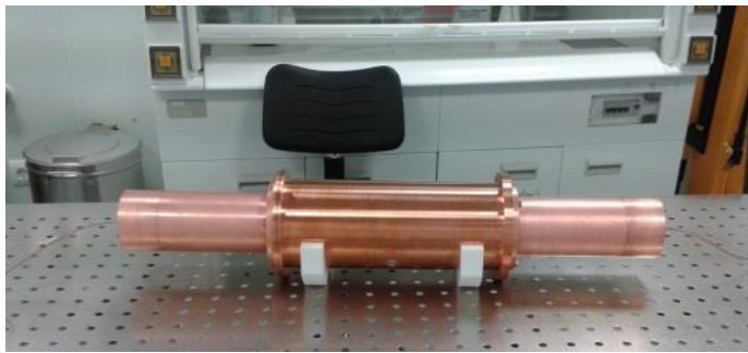
NaI(Tl) module assembly in the LSC Clean Room
