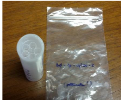
Acrylic sample + standards in the irradiation containers (one per sample)
