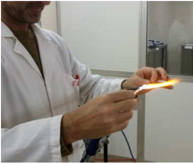
Preparation of the standards inside quartz vials
