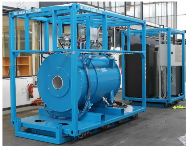
PUMA magnet and transport frame
