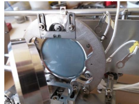
Side view: MCP + Phosphore screen
