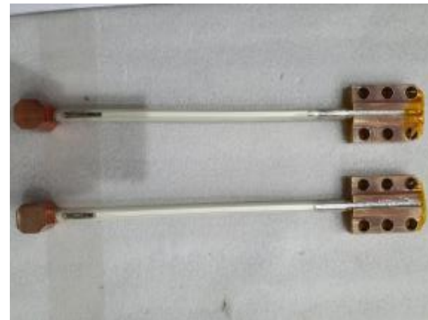
HTS current lead (performance test at 77K)
