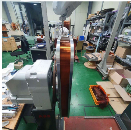
Quadrupole coil winding (automatic winding method)
