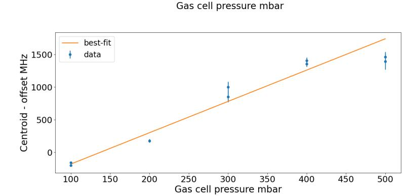
The broadening coefficient (T<sub>coll</sub>) and the shift coefficient  $(T_{sh})$  are calculated to be 8(2) MHz/mbar and 5(1) MHz/mbar.
