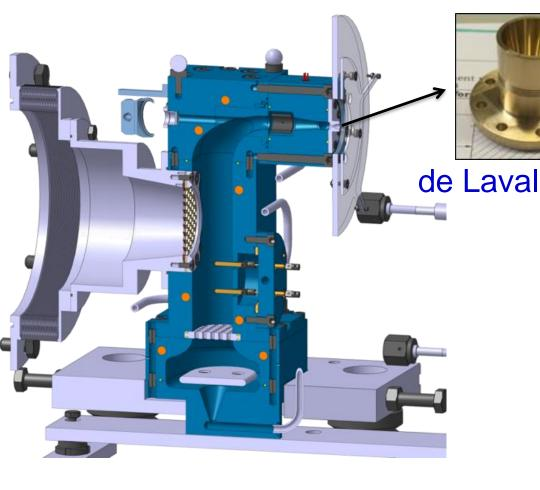
De Laval Nozzle creates a jet of atoms with narrow velocity distribution and low density thereby reducing temperature and collision rate.
