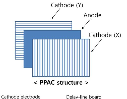
Position  $x = k(T_2 - T_1) + x_0$
