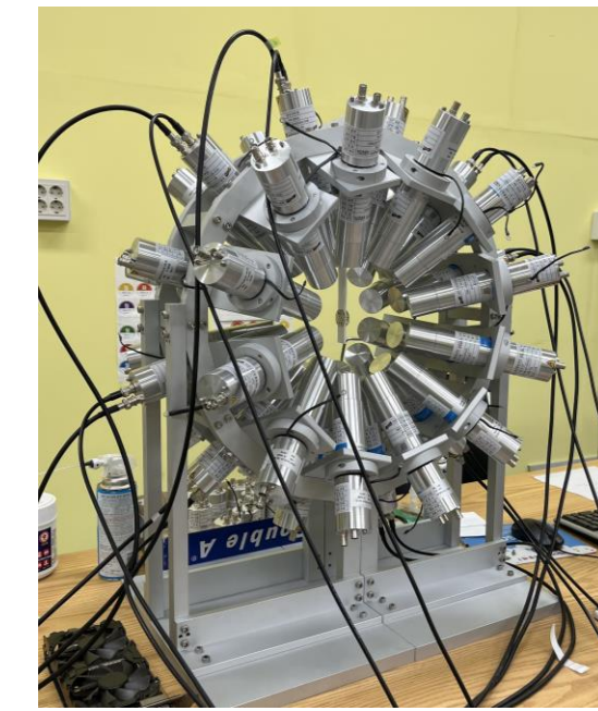
KHALA 36 ea. \phi 1.5'' \times 1.5'' LaBr 3 (Ce) developed by CENuM
