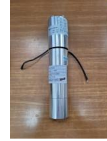
KHALA 36 ea. \phi 1.5'' \times 1.5'' LaBr 3 (Ce) developed by CENuM
