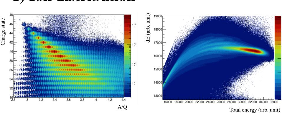
Projectile-like fragments are well identified for preliminary result (Q/ $\Delta$ Q ~ 80, M/ $\Delta$ M ~ 210)
