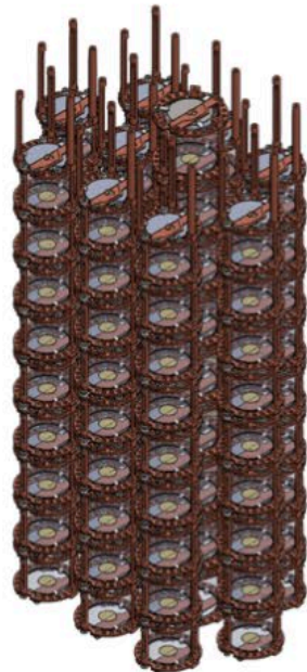
90 modules (~27 kg LMO) for the first stage
