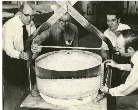
The first 32 inch diameter NaI(Tl) crystal. Pictured from left to right are Dr. Swinehart, Ed Jablon, Joe Knaus and Marko Stigol.
