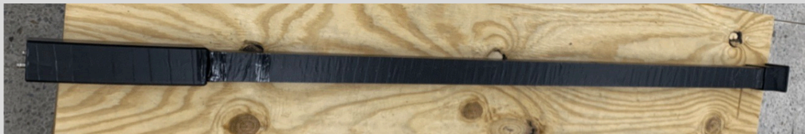
▲ A scintillator bar wrapped with teflon + Al foil + insulating tape
