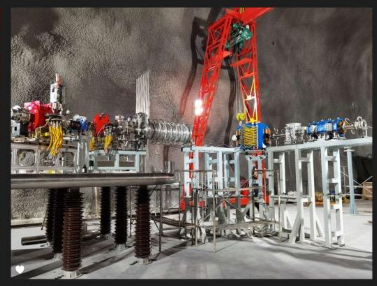
ECR source and acceleration tube
