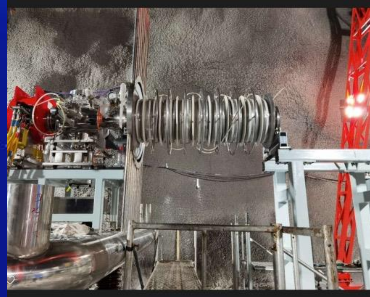
ECR source and acceleration tube
