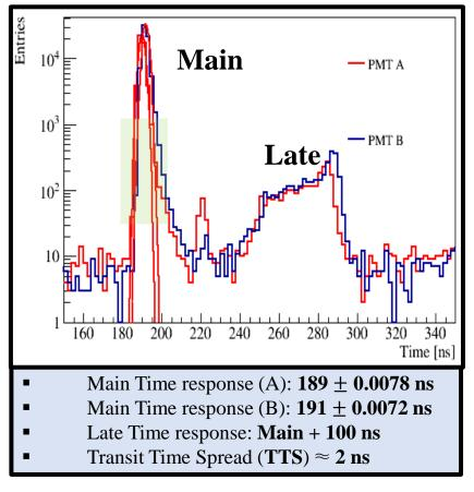
\*Time response: Trigger time – PMT falling time
