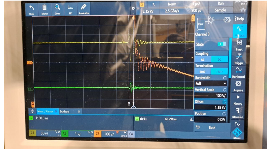
Ringin from the PDT after pulsing down
