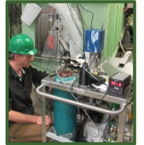
QWR cryomodule plasma processing (PP) (first time in-situ PP in low-beta cryomodules)
