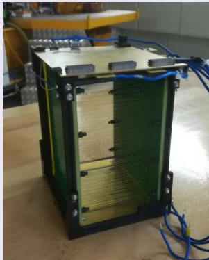
New tracker for the FPD ( THGEM technology)
