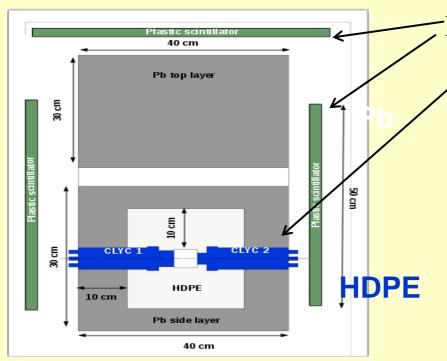
Muon detectors (plastic Scintillators)
