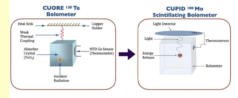
CUORE: no PID CUPID: PID allows to separate  $\beta/\gamma$  from  $\alpha$  events
