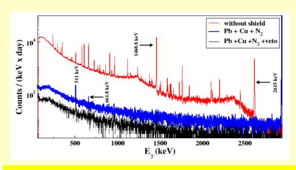
Sensitivity of the setup:  $\sim 1 \text{ mBq/g} (\sim 10 \text{ ppb})$
