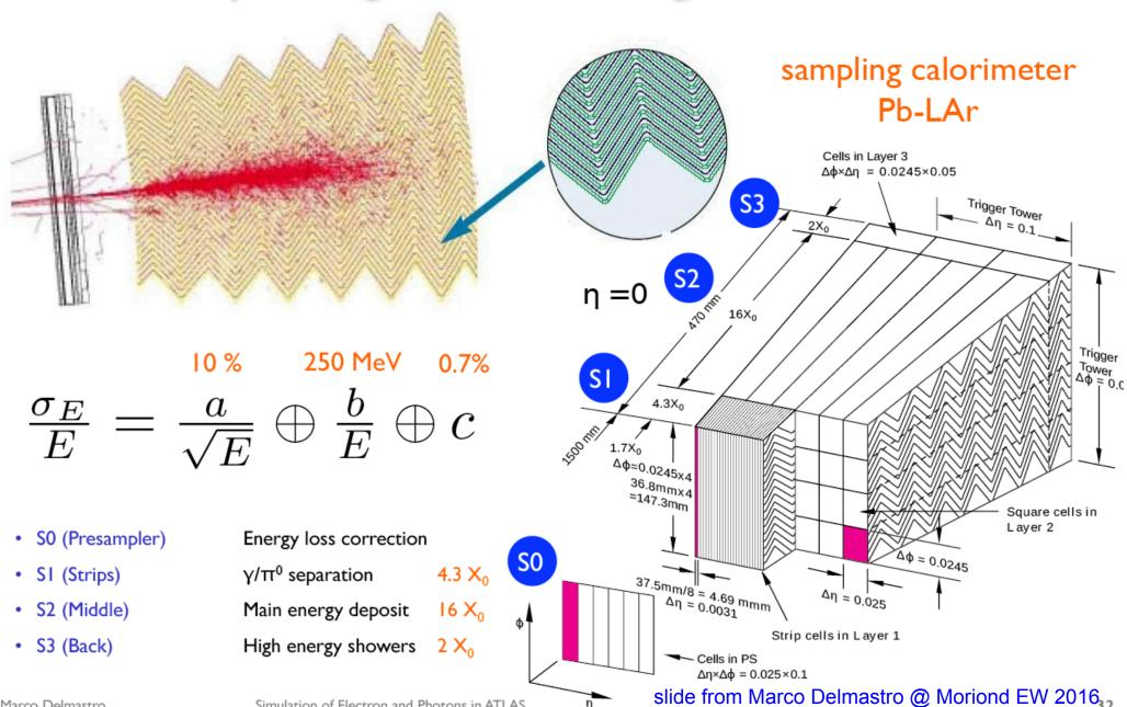
Simulation of Electron and Photons in ATLAS
