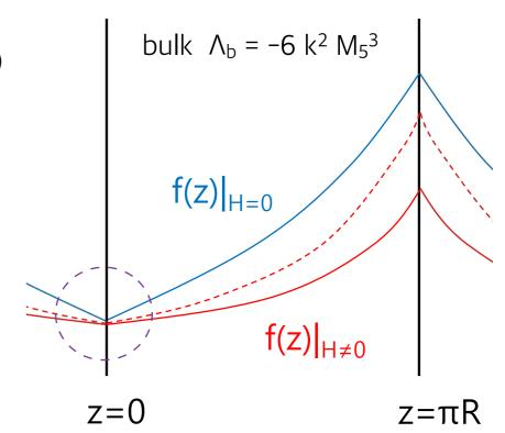
The smaller effective IR brane tension leads to weaker warping along the extra dimension.
